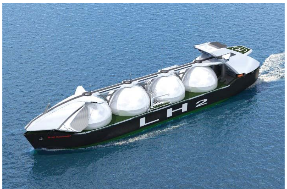
Large Liquefied Hydrogen Carrier developed by Kawasaki Heavy Industries
