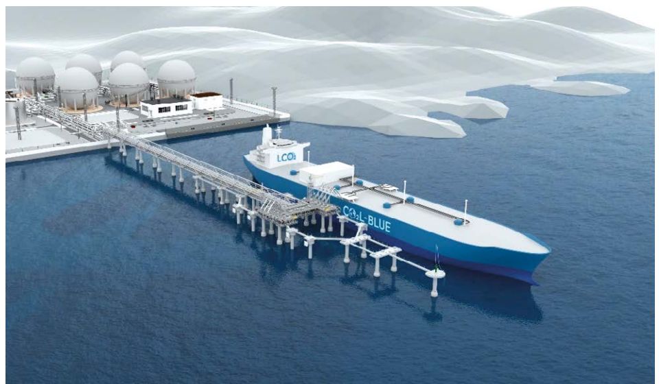
Large Liquefied CO 2 (LCO 2 ) Carrier developed by Mitsubishi Shipbuilding and NYK Line
