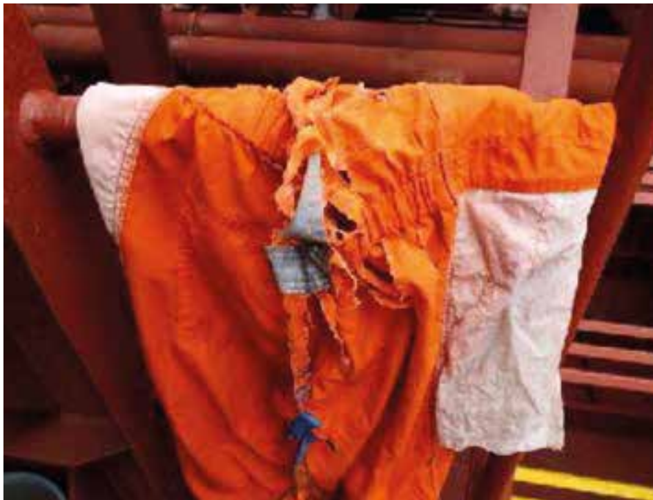
The coverall worn by the injured seafarer, showing how it was burned through by sulphuric acid
