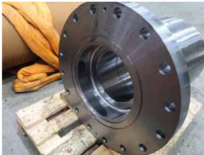
MarineShaft manufactured a new shaft coupling
