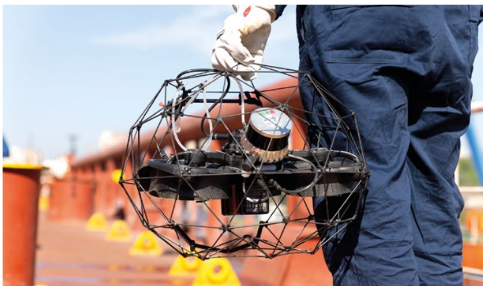
Flyability drone with a lighting system and protective cage. Image Flyability
