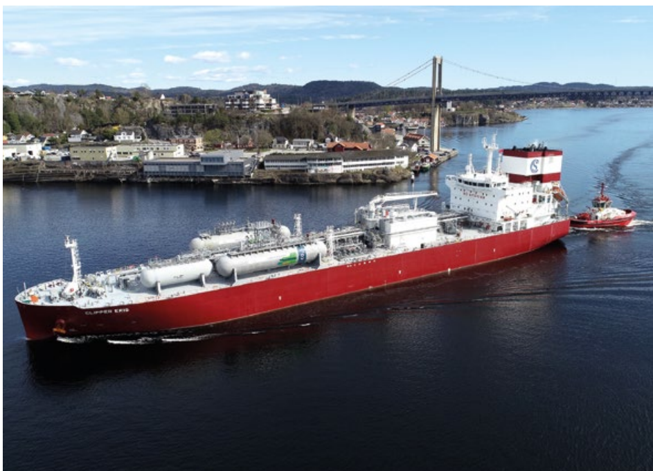
Solvang’s “Clipper Eris” with a CO 2 capture system and CO 2 tanks onboard
