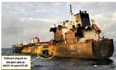
Hafnia Nile showing collision impact and subsequent fire damage. (Source: Hafnia Nile company and annotation by TSIB)
