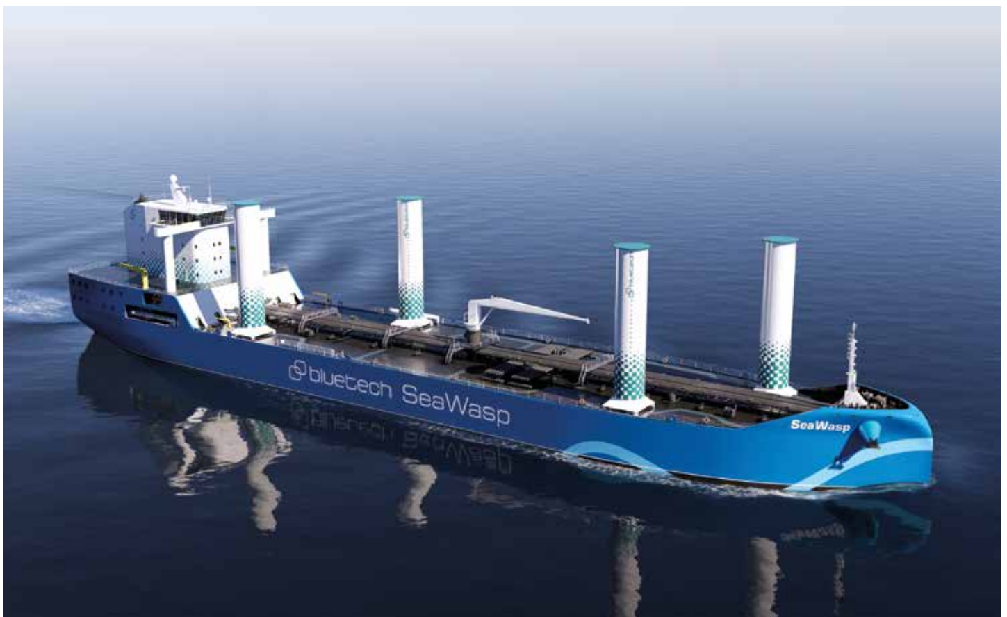
Digital rendering of Bluetech’s SeaWasp vessel concept equipped with four Norsepower Rotor Sails
