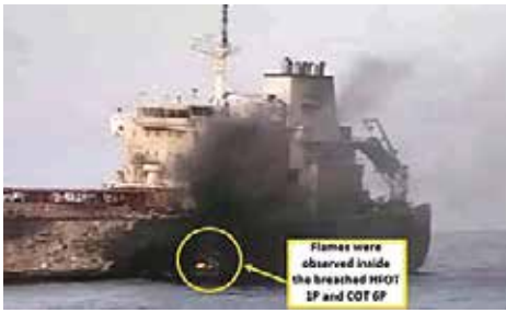
Photograph taken later in the day shows residual fire and smoke originating from Hafnia Nile's breached heavy fuel oil tank and cargo oil tank (Source: CI-Company and annotation by Transport Safety Investigation Bureau)
