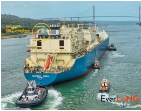
The carbon capture system (circled) fitted on an LNG carrier
