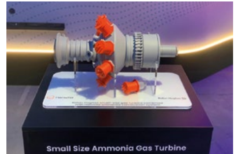
A model of the Baker Hughes / Hanwha Ocean ammonia turbine for shipping, generating up to 16 MW of power, enough for propulsion of a large vessel
