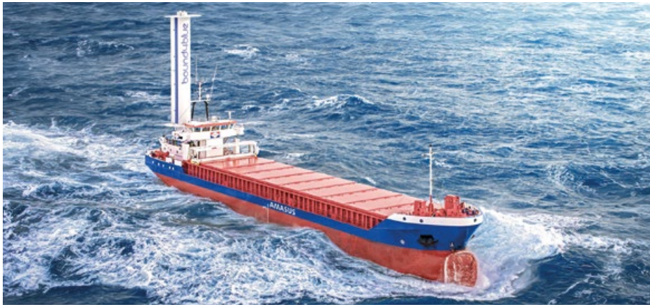
A suction sail installed on the Amasus short sea bulk carrier “Eems Traveller”
