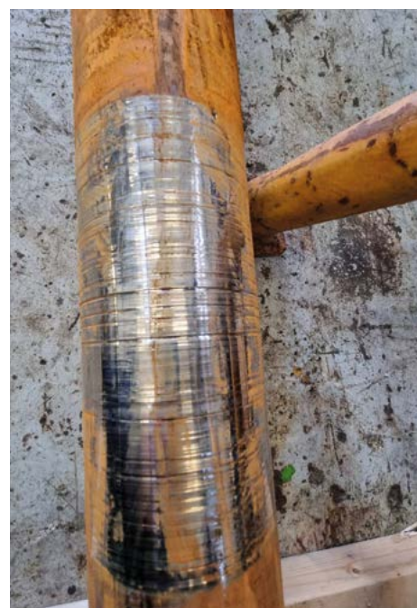
Corrosion on the shaft of MT Keilir – showing areas which needed repair
