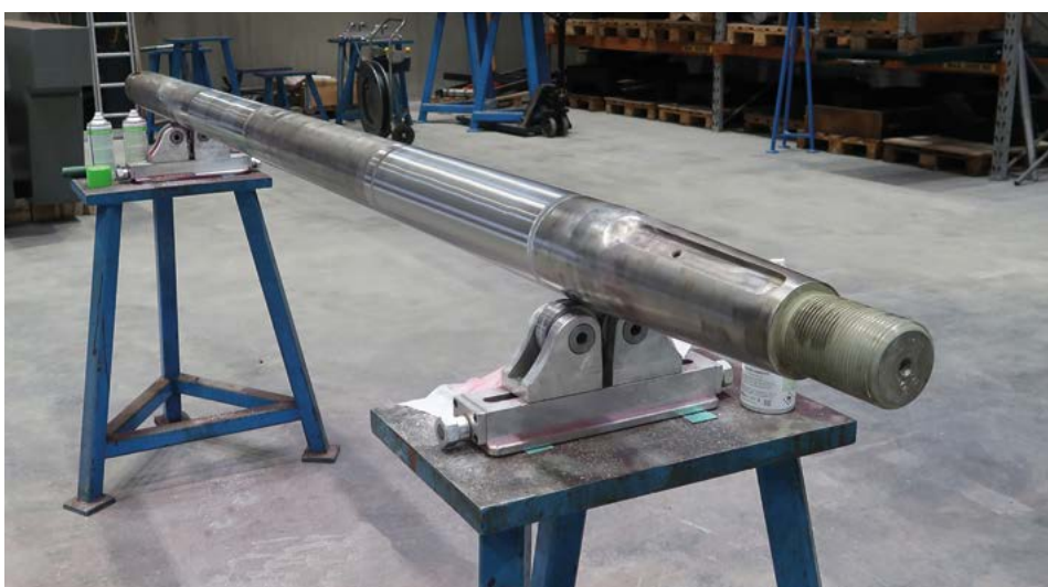
Finished shaft for MT Keilir with laser cladding completed
