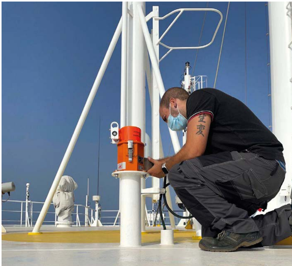
Sandvik Marine installs a voyage data recorder in Gibraltar
