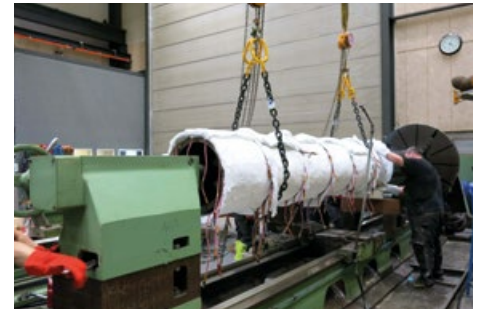
Heating the liner before shrink fitting
