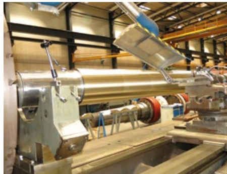
Checking the outer diameter of the liner
