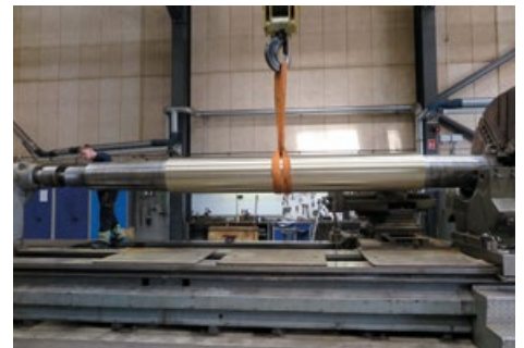
The shaft with the new liner, ready for delivery to the tanker
